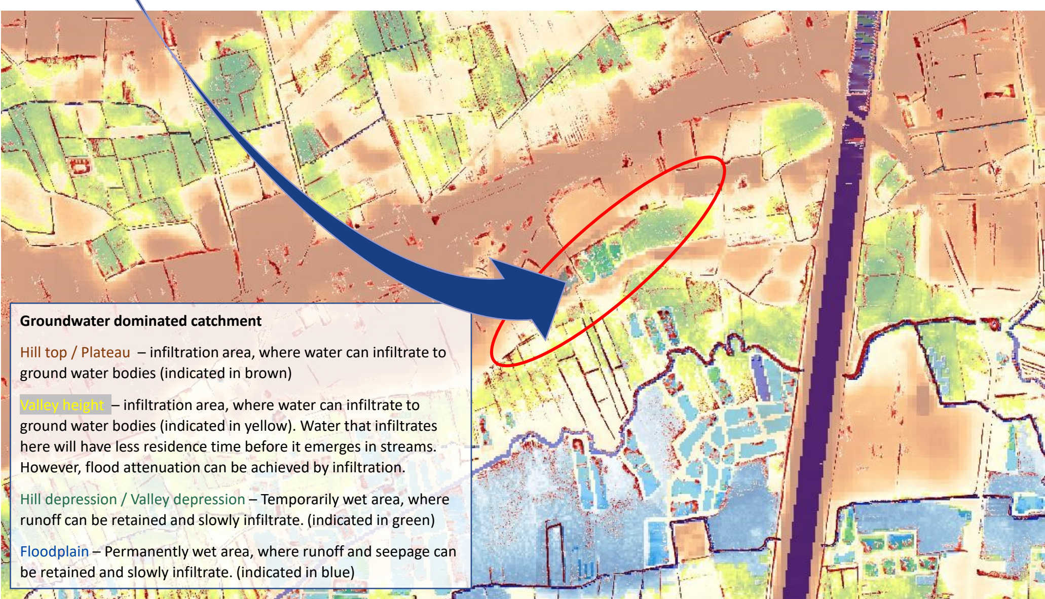
The water system map, applied to the demonstration site. The restored fens are situated in the blue-green zone. The restored deciduous forest edge and heathland are situated in the adjacent brown and green-yellow zones.
