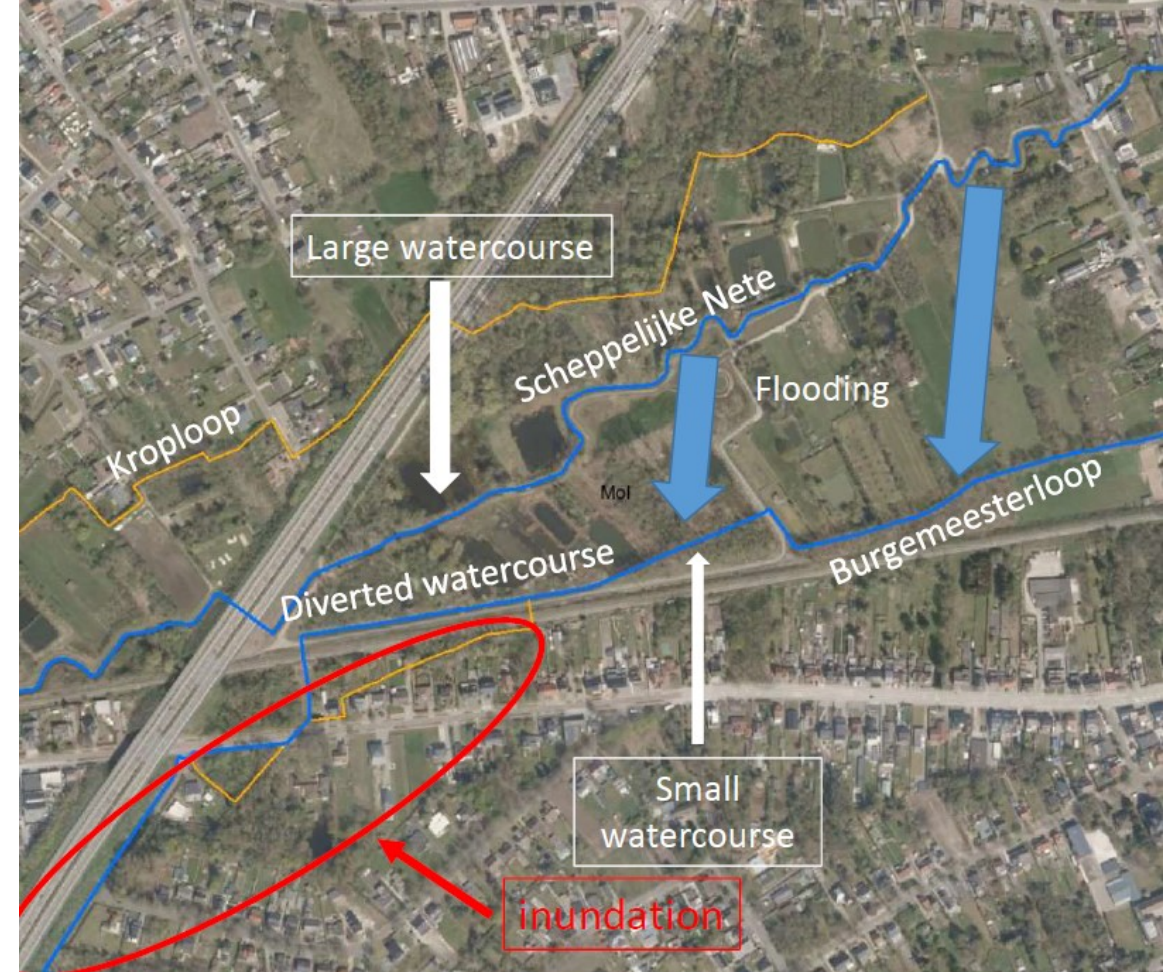
Indication water courses in the area and previous inundation problems. The restored floodplain and diverted water courses will help lower the chances for inundation downstream.
