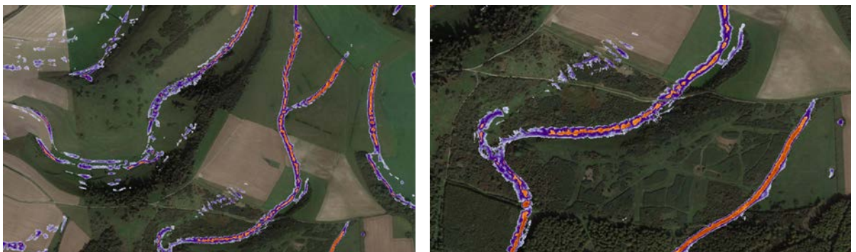
Figure 40 - Two sites in Friston Forest (left: east of Deep Dean and just north of Lullington Heath, right: Lullington Heath). Runoff attenuation areas and ditches follow clear valley lines. The darker zones visible in the left-hand image, which are identified as attenuation areas, could be on more acidic, slightly less permeable soil and so represent different seepage patterns than the thin chalk soils on most of the area.
